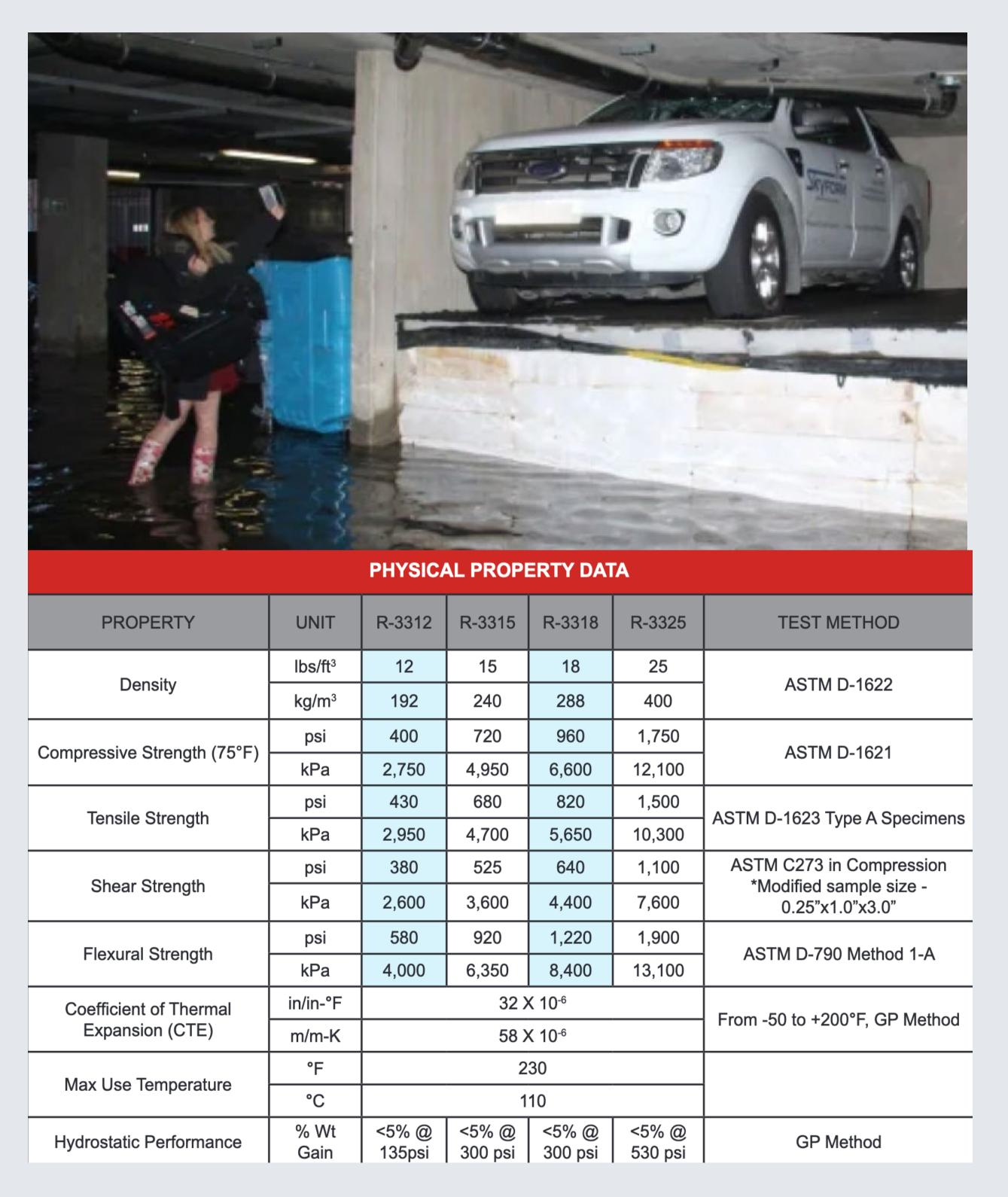
The image shows how the foam performs underextreme conditions. The rising flood water trapped this car in a corner and the buoyancy force crushed the roof. This is one indicator of how tough this foam really is.
